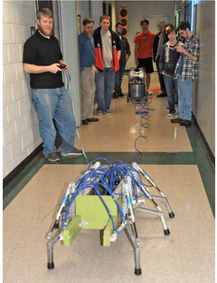
Last semester General Engineering Technology students in a senior Hydraulics and Pneumatics class explored pneumatics and PLCs (Programmable Logic Controllers) by building a six-legged walking machine (Hexapod), pictured here, powered by pneumatics and controlled by a PLC.
